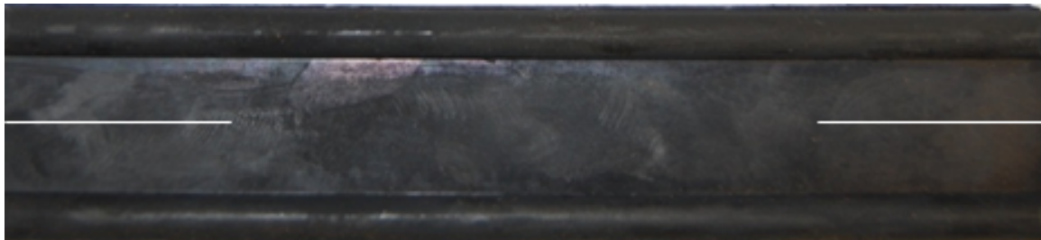
Figure 7.1 Pure shear specimen used for FCG testing
