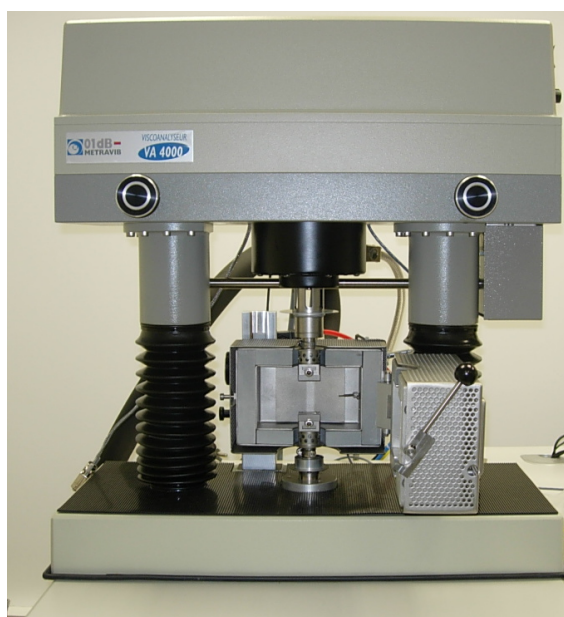
Figure 3.3 Dynamic Mechanical Analyzer (Metravib VA 4000)
