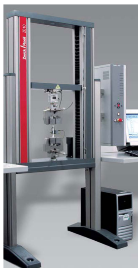
Figure 3.2 Universal Testing Machine (Zwick Z010)
