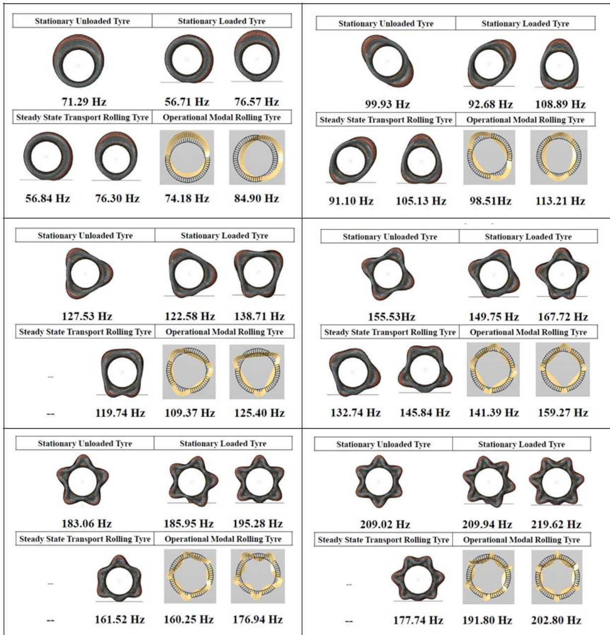
Figure 3.17 Mode shape comparison among various tyre conditions
