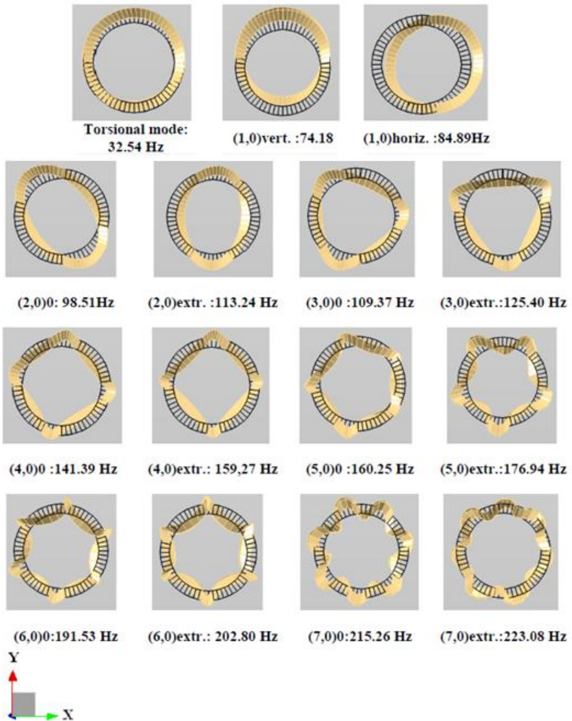
Figure 3.12 Operational modal parameters obtained from straight cleat impact test
