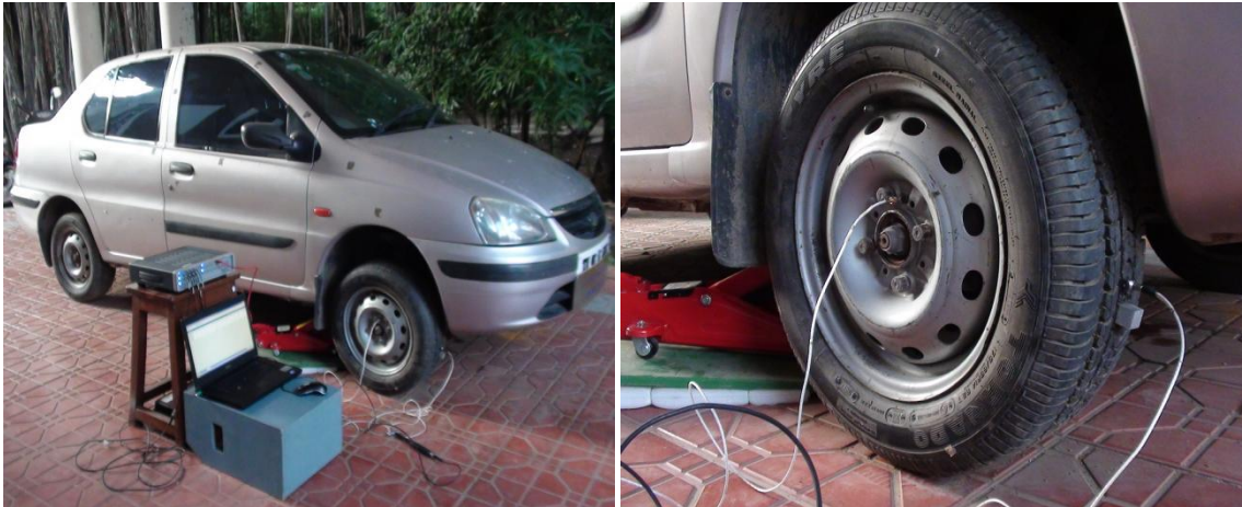
Figure 5.4 Experimental set up of front tyre wheel assembly for tyre transfer characteristics by in-situ method
