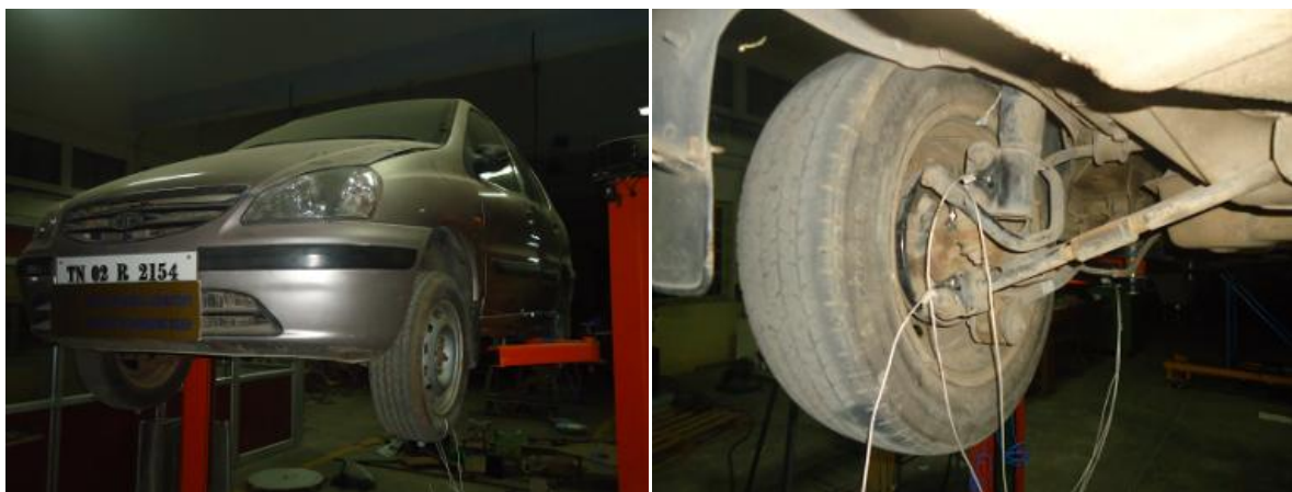
Figure 5.2 Laboratory experimental set up for full vehicle system (TV)
