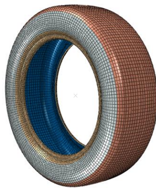
Figure 3.1(b) Tyre FE model
