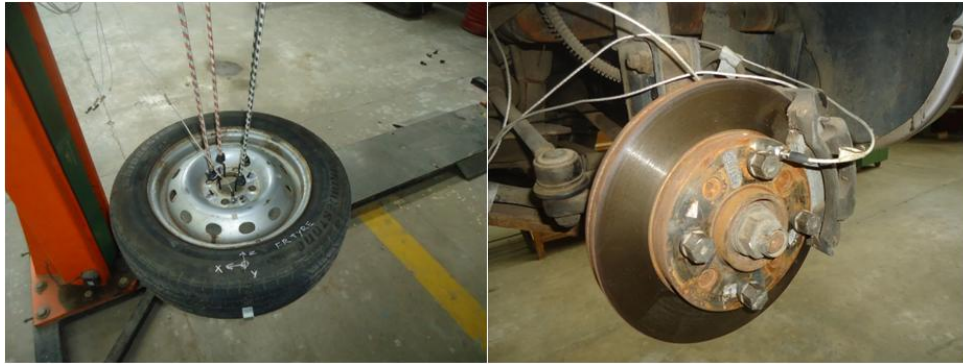
Figure 5.6 Position of accelerometers for free velocity method
