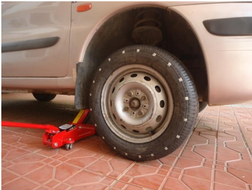
Figure 2.13 Spindle fixed condition of unloaded tyre for experimental modal analysis
